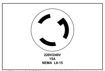
Figure 1. NEMA 6-15 220V/15A connector.
